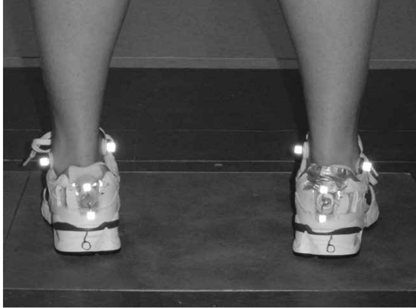
Figure 4 — Posterior view of the shoes with heel counter removed and the custom heel markers
