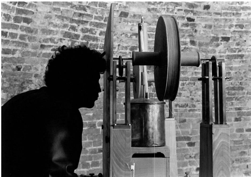
FIGURE 5: A sequence in the restaging of James Joule's paddle-wheel experiment with a replica. The experimenter is reading a thermometer scale while hiding behind a wooden shield so that the radiation of body heat will not interfere with the thermometer placed in the water-filled copper vessel. Photo by Norbert Gerdes, Oldenburg, Germany.
