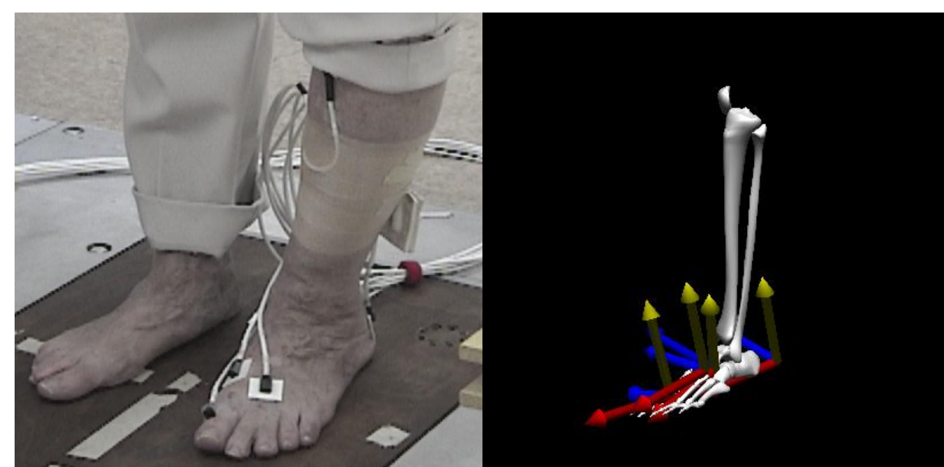
Figure 1. In vivo kinematic model and subsequent subject-specific anatomically based co-ordinate systems used to assess in vivo foot motion during barefoot walking
