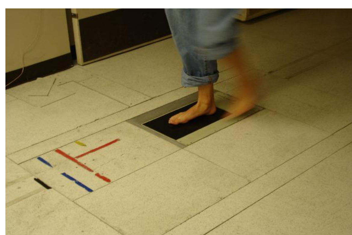
Figure 1: Peak pressure, contact area, and pressure-time integral were determined using an EMED plantar pressure system. A 40/60 split of the foot was used for data collection to separate the hindfoot from the midfoot and forefoot.
