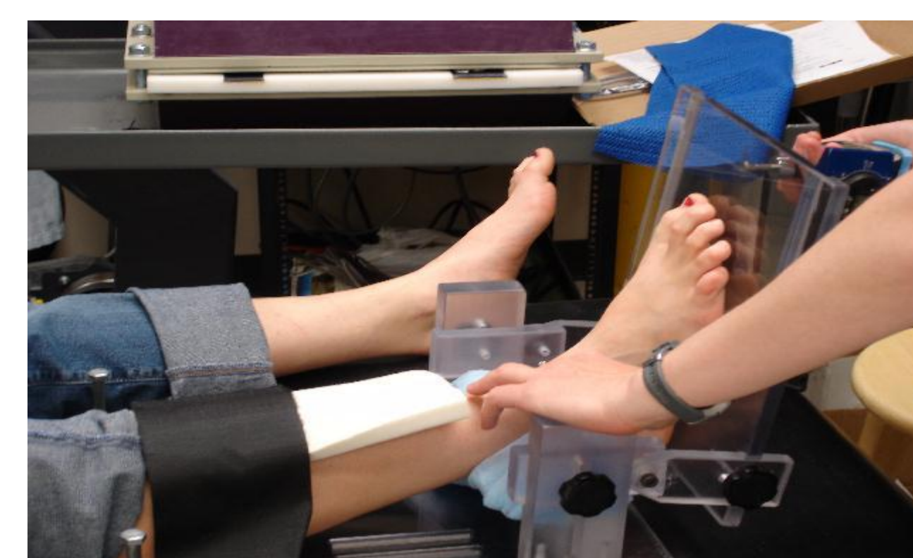
Figure 4: lowa Ankle Range of Motion device was used to measure peak dorsiflexion and ankle stiffness. Torques of 10, 15, 20, and 25 Newton-meters were applied about the ankle joint while a digital inclinometer was used to measure the angle of dorsiflexion.
