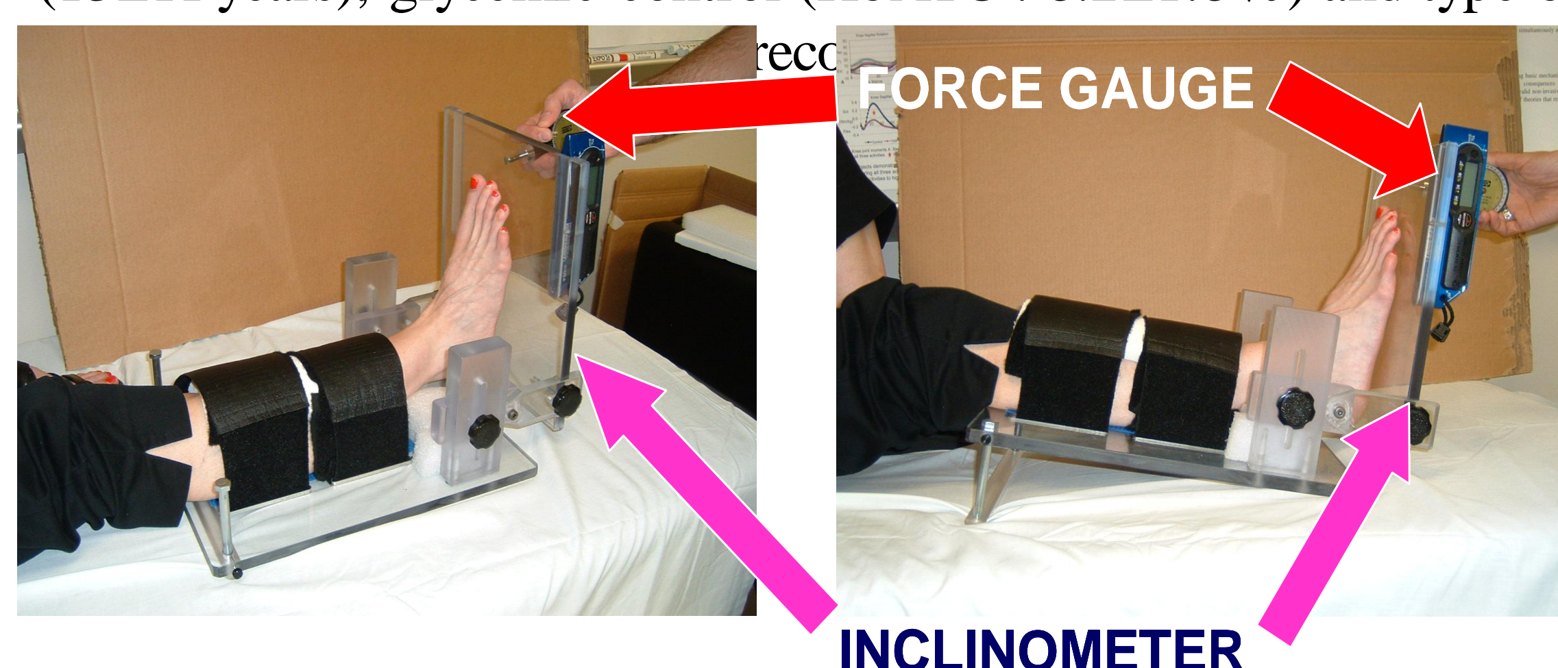
Figure 1: Custom device used to measure ankle dorsiflexion while applying torques of 15.27, 20.37 and 25.46 Nm.
